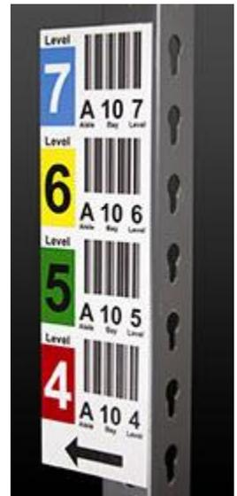
The barcodes used for shelf locations in warehouses should be at least 3 inches wide with three eighths of an inch of white space either side and have 20 mil resolution barcodes so they are easy to scan from a distance. They should be placed on the uprights of racking one above the other at about eye level, as shown below:
