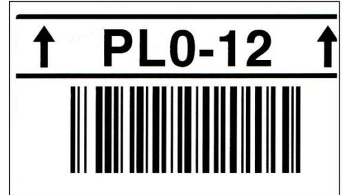
It consists of a one dimensional barcode, which contains the code for the location with the same code in human readable form. It may also contain arrows and other indicators to enable the selection of the correct barcode to scan for a shelf.
