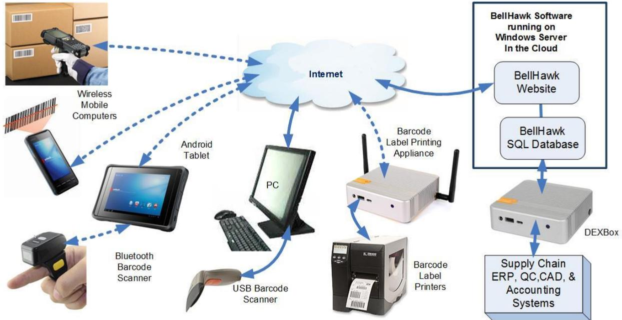
The BellHawk software consists of a specialized website and a SQL Server database that run on a Windows Server computer. All user interaction is performed using web-browser based devices.
