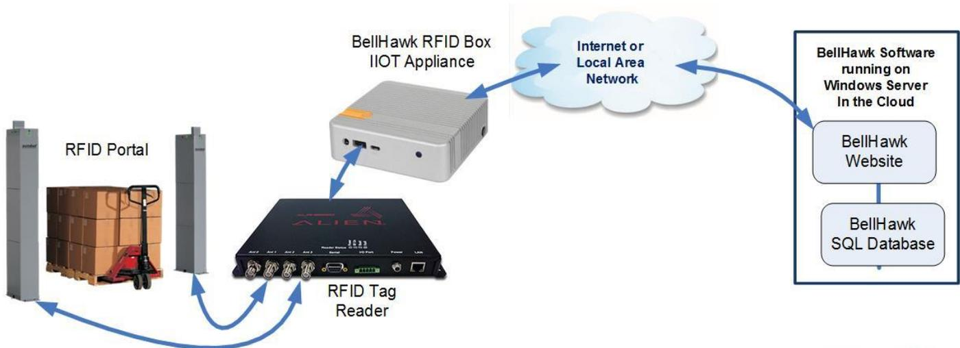
In BellHawk, individual items as well as containers of material can be tracked using "license-plate" RFID tags as well as tracking barcodes. In practice, many such containers may have combination RFID tags (1) embedded in combination barcode labels (2) printed out using the BellHawk Barcode Label Printing (BLPA) I/IOT appliance, as shown at right.
