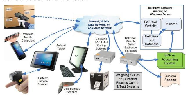
The BellHawk data collection software consists of a specialized website and a SQL Server database that run on a Windows Server computer. All user interaction is performed using webbrowser based devices thereby avoiding the need to install custom software in each device.
