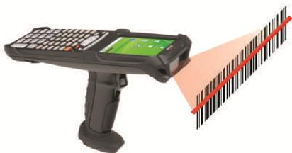
In doing barcode inventory tracking we will typically attach a “license-plate” tracking barcode to a finished goods item or a container, such as a box or pallet, of finished goods. Then we associate the tracking barcode with the part number for the item or items within the container and record the quantity in the container and its location.
