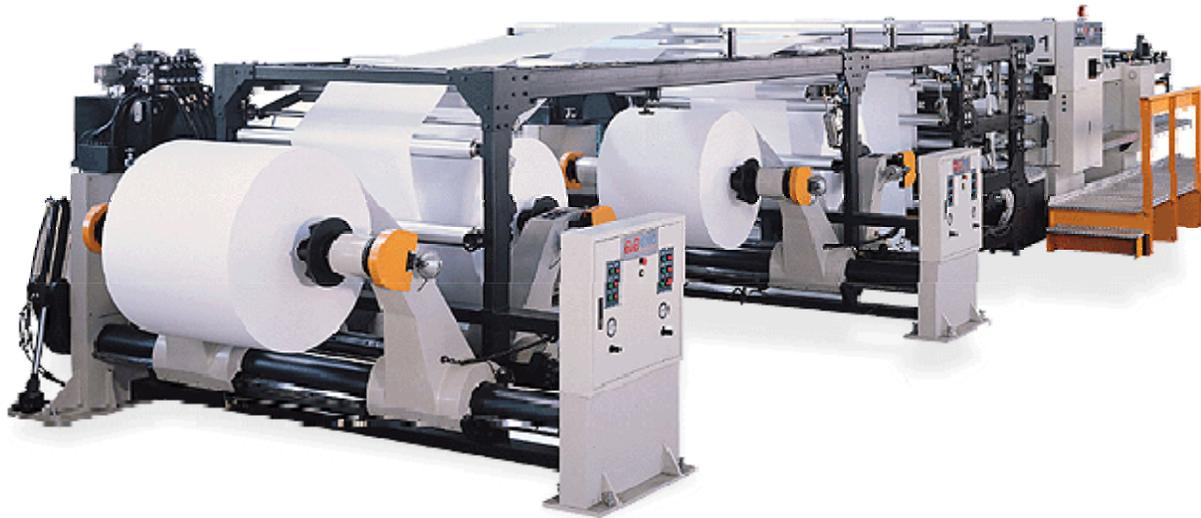
This company purchases large rolls of paper, plastic and aluminum foil and then coats these in a wide variety of colors to meet the specific packaging needs of clients. After coating, the rolls are slit and then sheeted and boxed, according to the needs of each customer order. Almost all of their products are made to order, with typical runs lasting from a few hours to weeks.
