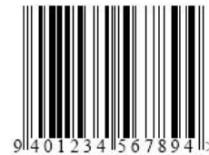
EAN-13 symbol EAN/UCC-13 structure
