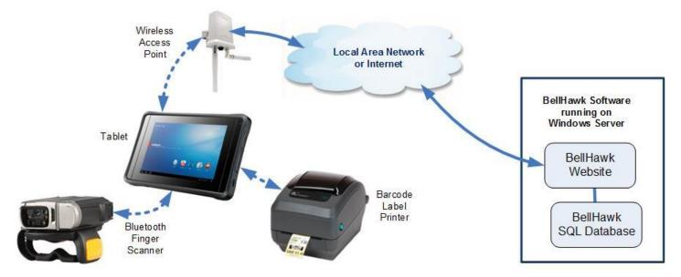
The BellHawk software runs on a Windows Server computer, which is typically in the cabinet manufacturing facility, but can be in the "Cloud". BellHawk consists of a specialized website and a SQL Server database. The website can be accessed by any web-browser based device over the Internet or the shop's local area network.
